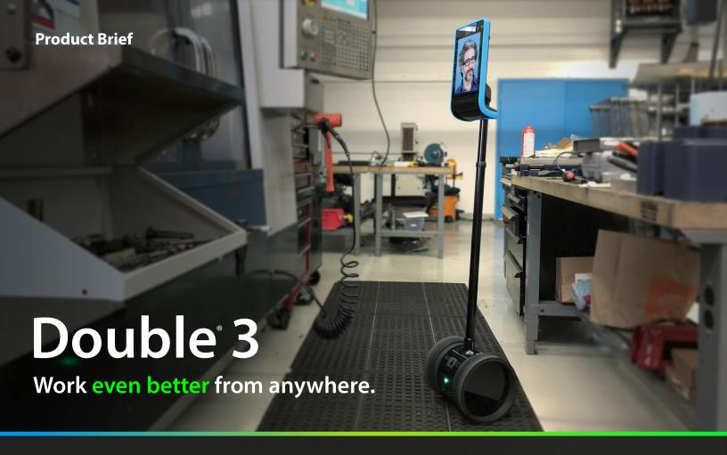
Double 3 is a self-driving, two-wheeled videoconferencing robot that revolutionizes the way you work or learn remotely.
