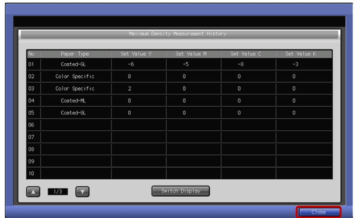
**Note:** If there is a large jump in values between the history data of the same **Paper Type**, it may be necessary to turn off **CDC** and repeat **Density Balance** and **Max Density Initial Adjustment**.
