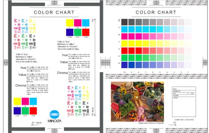
Check the overall condition of the image print area by printing the following test pattern.
