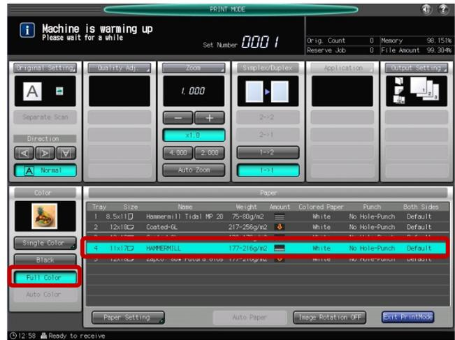
12 prints are output for CMYK colors, as well as, halftone prints of R-G-B and processed black. If necessary, print Test Pattern +53 for specific colors at varying densities to further identify image density issues.
