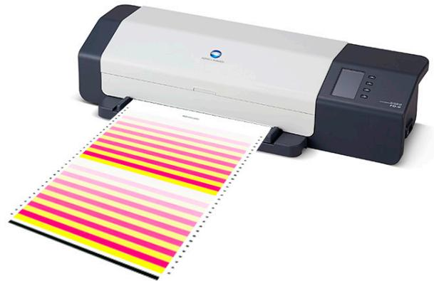
4. On an **i1-iSis XL**, align the **Density Balance Chart** to the **left side** of the entrance, feed the chart in with the registration (black) bar in first; making sure to push the sheet far enough into the device for it to grab the chart.
